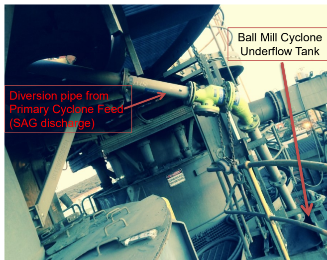
Figure 5: Diversion of the SAG discharge (primary cyclone feed) to the ball mill
